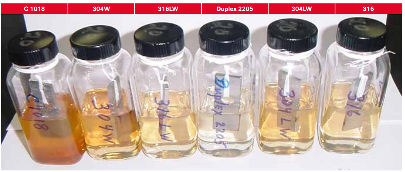
Figure 5: Test coupons half above and half below GeoBrom® HG520 after 90-day exposure at 20 °C
