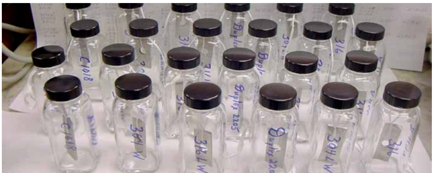
Figure 3: Test coupons before GeoBrom HG520 charged and before 90-day exposure
