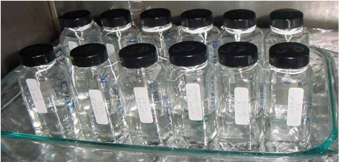
Figure 4: Test coupons before 90-day exposure at above and half below surface in GeoBrom® HG520
