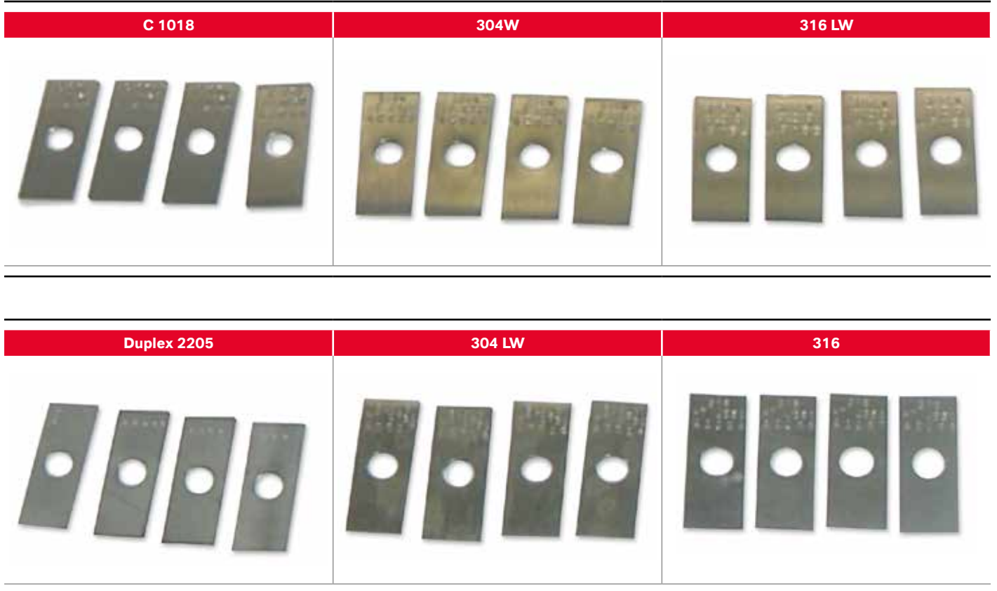
Figure 2: Test coupons before 90-day half above and half below surface exposure
