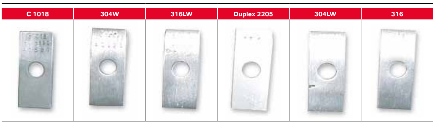
Figure 15: Test coupons half above and half below GeoBrom® HG520 after 90-day exposure at 50 °C after cleaning
