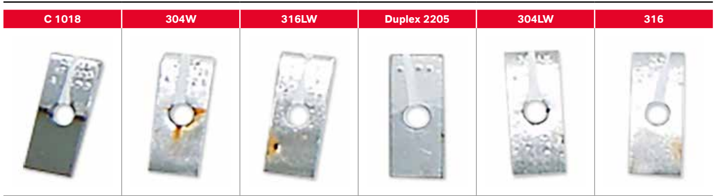
Figure 6: Test coupons half above and half below GeoBrom® HG520 after 90-day exposure at 20 °C
