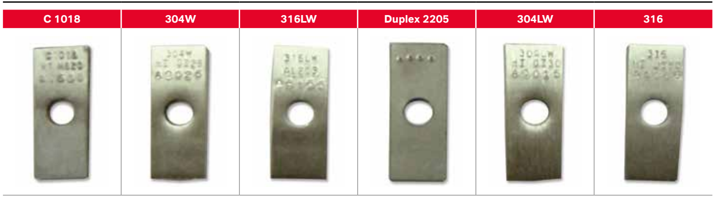
Figure 10: Test coupons half above and half below GeoBrom® HG520 after 90-day exposure at 20 °C after cleaning
