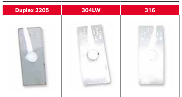
Figure 8: Test coupons before cleaning after 90-day exposure at 20 °C in GeoBrom® HG 520
