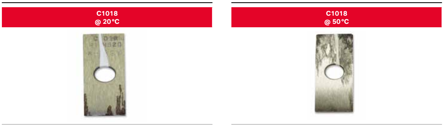
Figure 5: C1018 coupon after 90-day above surface exposure at 20 °C and 50 °C (before cleaning)
