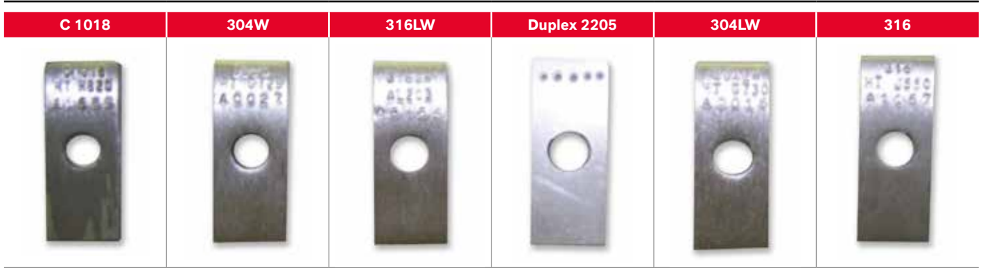
Figure 6: Test coupons after 90-day above surface exposure at 20 °C removed from test bottles (after cleaning)
