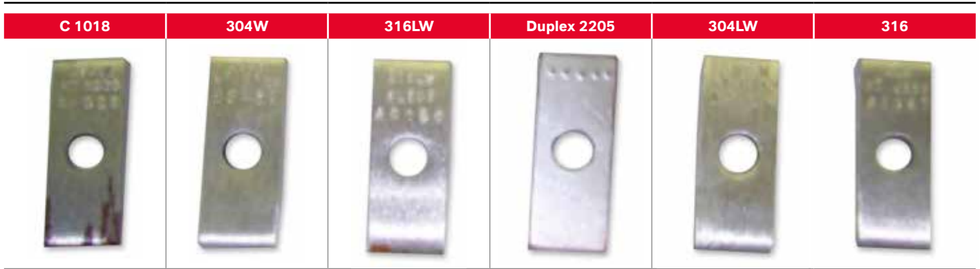
Figure 4: Test coupons after 90-day above surface exposure at 20 °C removed from test bottles (before cleaning)
