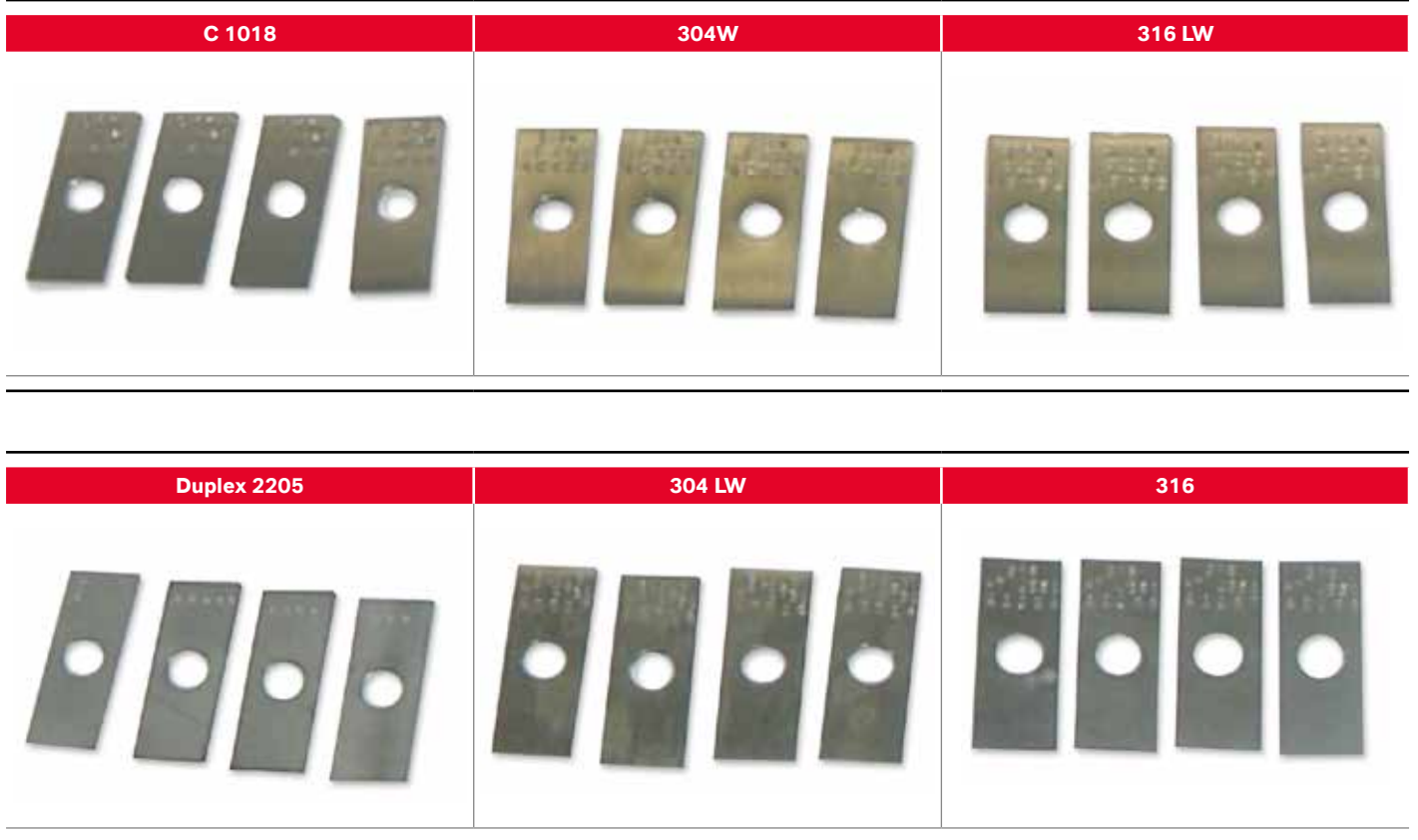
Figure 2: Test coupons before 90-day above surface exposure at 20 °C and 50 °C
