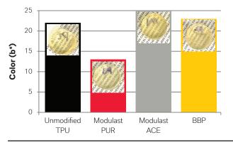
In contrast to BBP, Modulast PUR significantly improves color in the final TPU, while also improving the HS&E profile.
